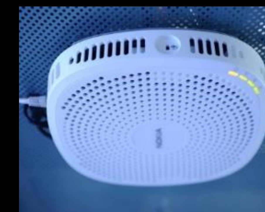
LTE small cell @3.5GHz
